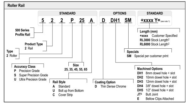
Y = Distance from end of rail to center of first mounting hole, Y1 = Y2 unless specified.
