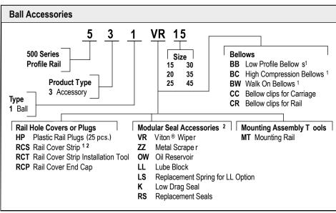
1. Bellows and rail cover strip must include length at time of order. Example: 531BB15 + 1000mm. See page 154 on how to calculate bellows length. 2. Cover strip not available in combination with stainless steel.
