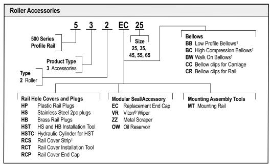
1. Bellows and rail cover strip must include length at time of order. (Example: 532BB35 + 1000 mm). See page 154 for how to calculate bellows length. THOMSON
