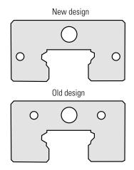
OW oil reservoir lubrication plate eliminates the need for a routine maintenance schedule, assures lubrication gets to the required points, can be refilled if required. I usually doubles the gap between service cycle. The Type 431 OW oil reservoir can be easily installed in conjunction with other optional modular accessories providing an easy upgrade to the standard seals. These can be easily installed on-site in the field or can be supplied from the factory.
