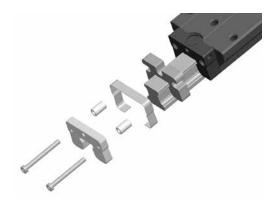
The self-lubricating Lube Block option offers maintenance free operation and enhanced protection for a broad range of applications. It offers:
