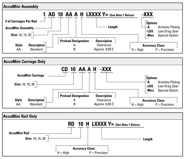
1. Y= Distance from end of rail to center of 1st mounting hole
