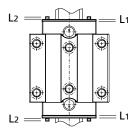
L1 – scraper thickness, L2 – max. screw head stickout
